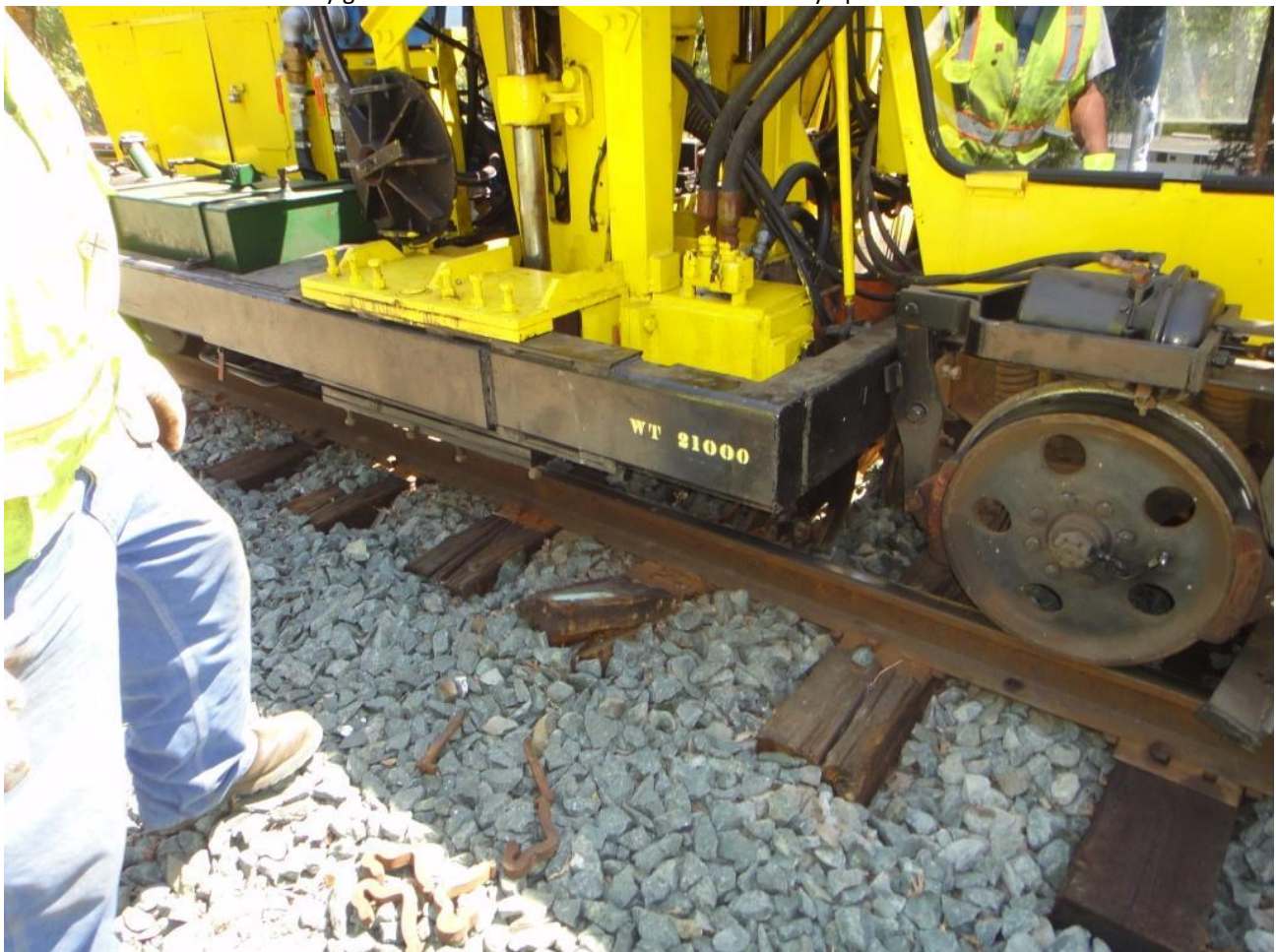
The tie-shear's "kickers" kick-out sliced tie-ends
